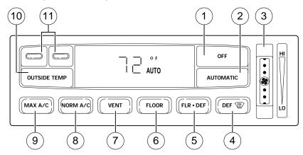
1. **OFF:** Outside air is shut out and the fan will not operate.
